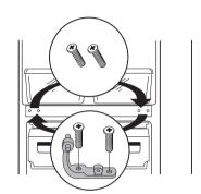
Unscrew the retaining screw for the self-closing mechanism on the bottom of the fridge compartment door.
